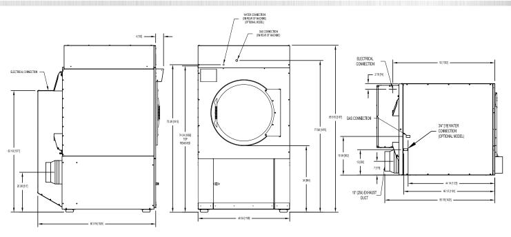
\*Control location on this model varies depending on the control option selected. Drawings shown display placement for O-series control.
